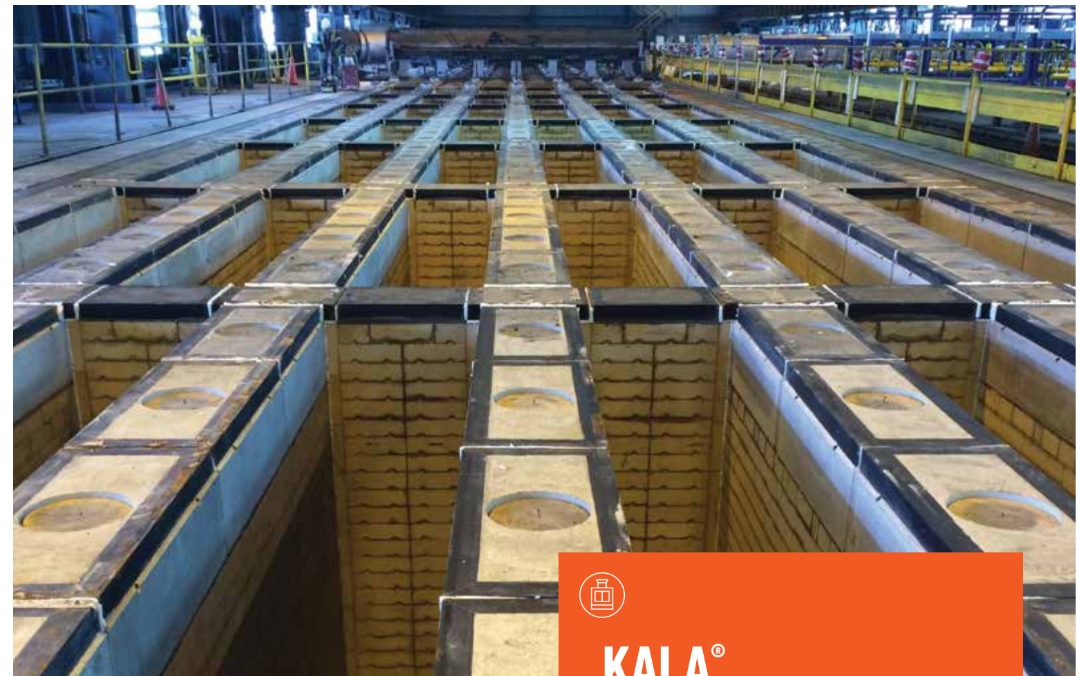
ABOVE: HWI's KALA® brick installed in a carbon anode baking furnace at a large smelting facility.
