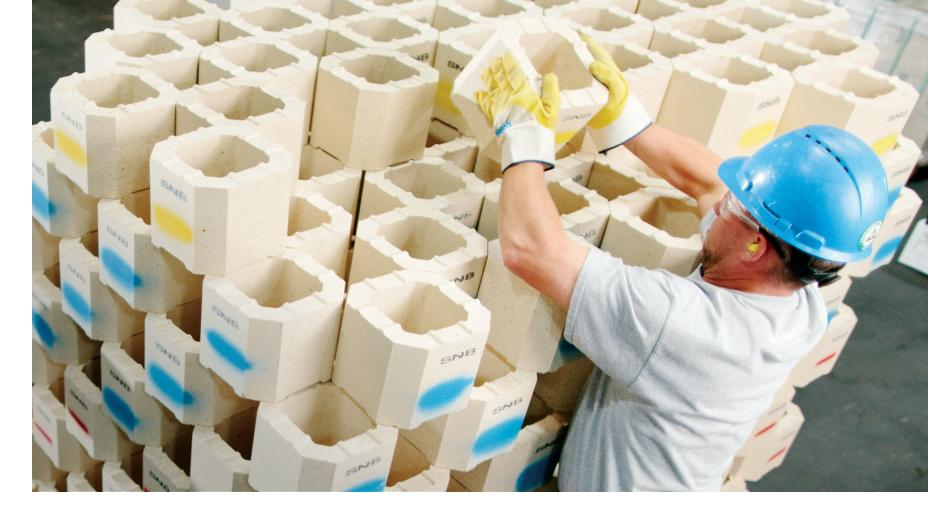
Various checker designs are available to suit your needs, including conventional settings, HPC (chimney type), and the HYDE Checker. All modular checker settings available from HWI can be designed with horizontal clean-outs where appropriate. In addition, all modular checker settings are color coded to height groupings to provide excellent stability.
