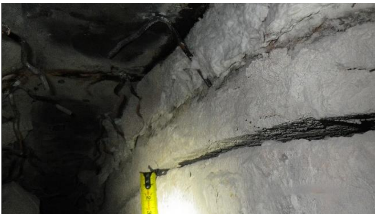
Figure 8: Thermal reactor hot face bricks along top center have sagged downward resulting in an open gap between hot face and backup layer.
