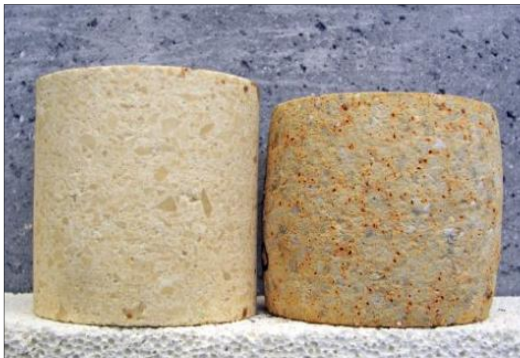
Figure 2: Comparison of refractory samples before (left) and after (right) a creep test.
